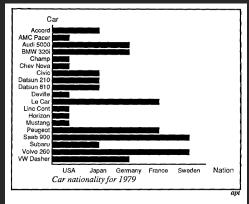
Fig. 11. Incorrect use of a bar chart for the *Nation* relation. The lengths of the bars suggest an ordering on the vertical axis, as if the USA cars were longer or better than the other cars, which is not true for the *Nation* relation.
