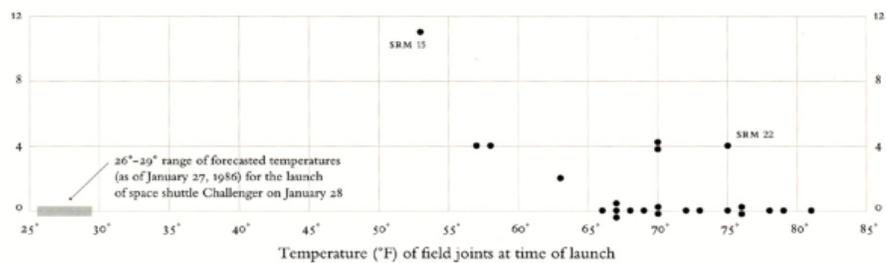
Visualizations drawn by Tufte show how low temperatures damage O-rings [Tufte 97]
