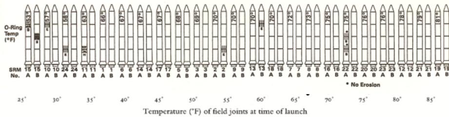
Visualizations drawn by Tufte show how low temperatures damage O-rings [Tufte 97]
