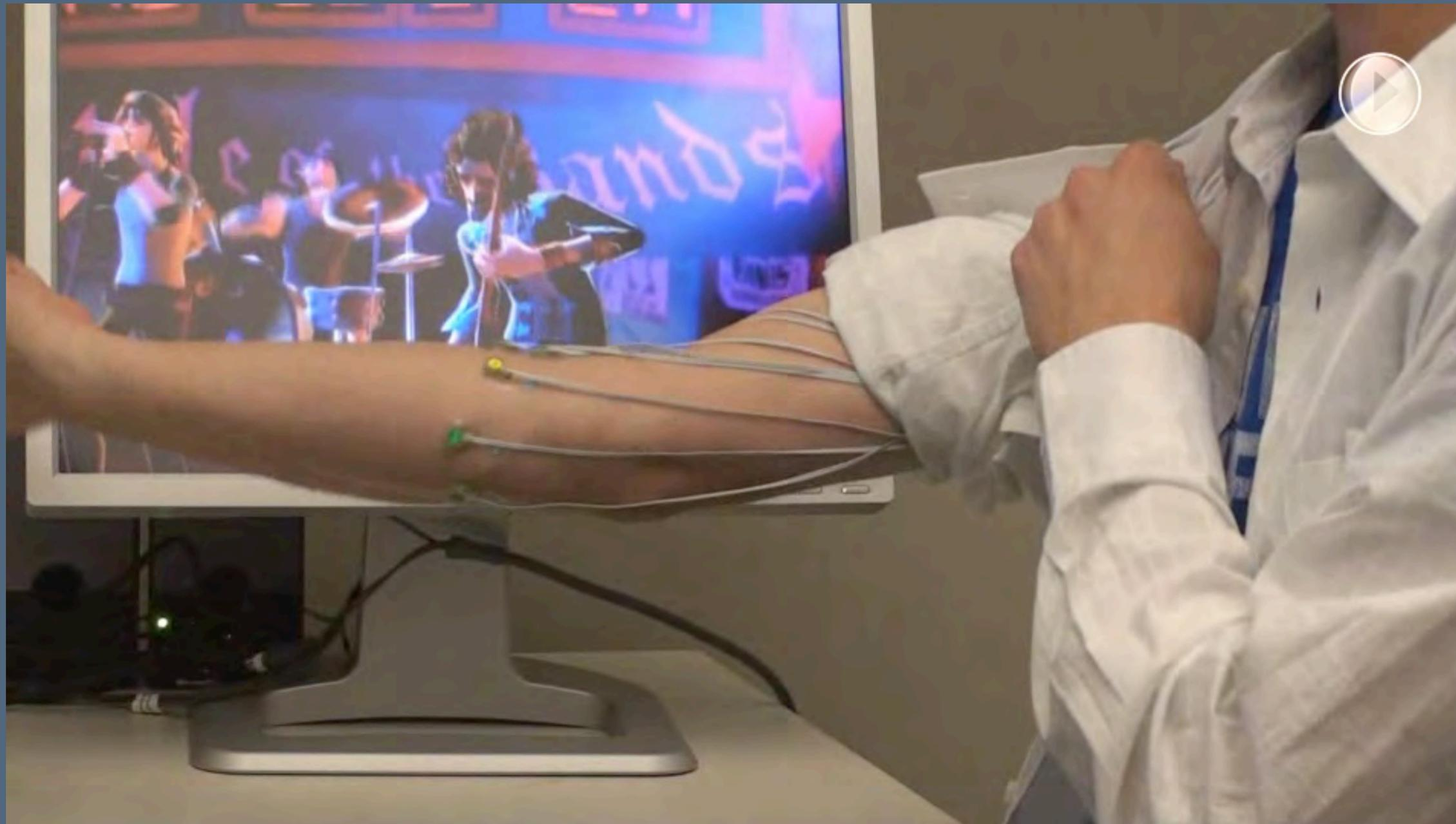
Recognize hand gestures with on-body instrumentation
