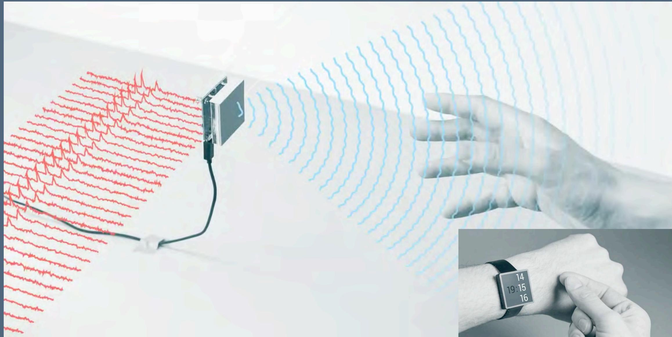
Example: radar (radio wave reflections) scatters a wide beam and captures responses from many different parts of your hand as the waves reflect off of it
