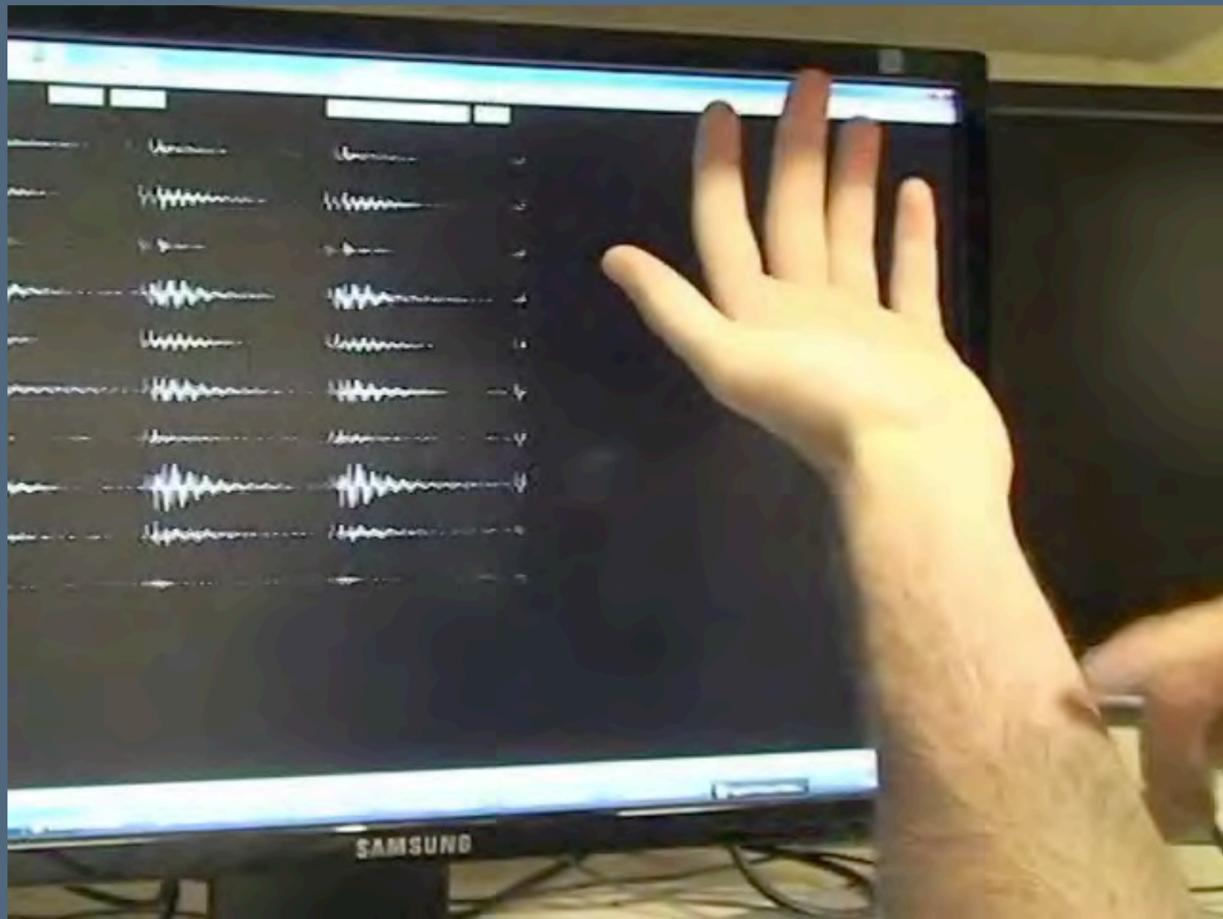
Example: treat vibration data as audio data and derive similar features (FFTs, average amplitude of each sensor, amplitude ratios between pairs of sensors)
