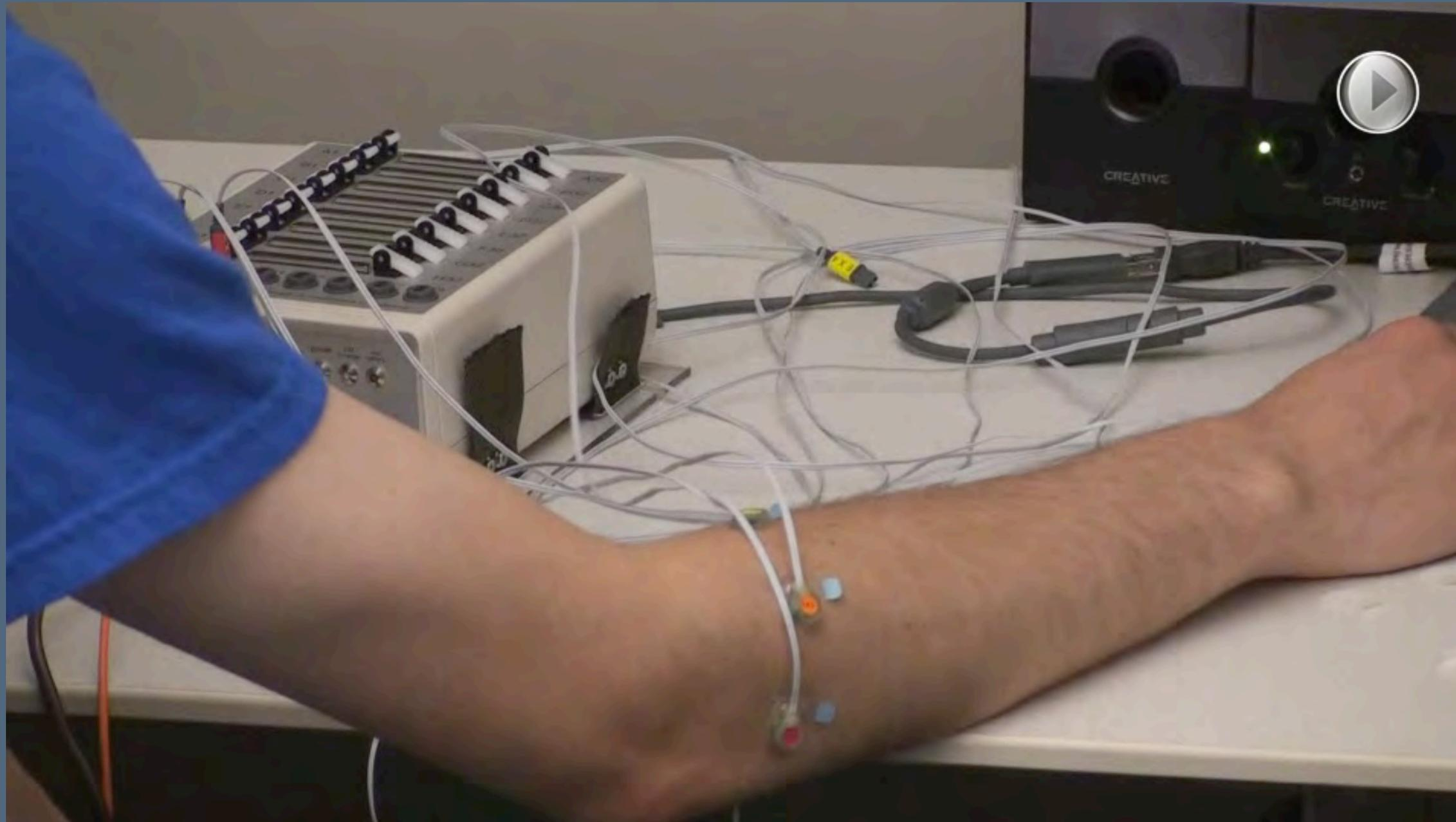
Example: attach EMG sensors in a band around your arm: forearm electromyography
